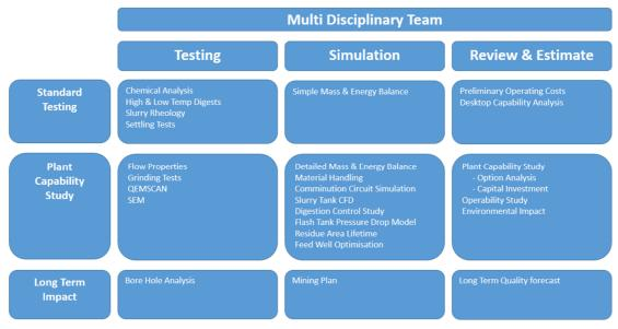
Figure 1. Bauxite Testing Protocol.
